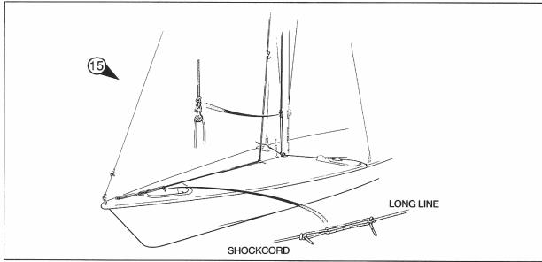
Attach the spinnaker pole uphaul/down haul line as shown, (Fig 15) .
