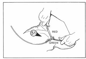
\* Identify the corners of the spinnaker and attach to the end of the sheet using a suitable knot. (Fig 52) ► . Red to port and green to starboard.
