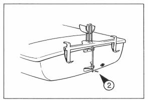
\* Detach rear mast support (if fitted) by removing 'R' clip (fig 2) ▼.
