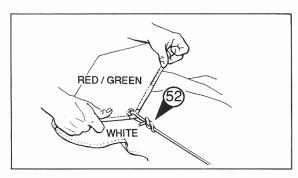
\* Attach the spinnaker downhaul line to the recovery patches on the inside of the spinnaker as shown. (Fig 53) .
