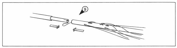
\* Take the top mast section (Part B) and slide into bottom mast (Part A) making sure the luff Igroove is in line and the sleeve is fully pushed home. (Fig 9) 4.
